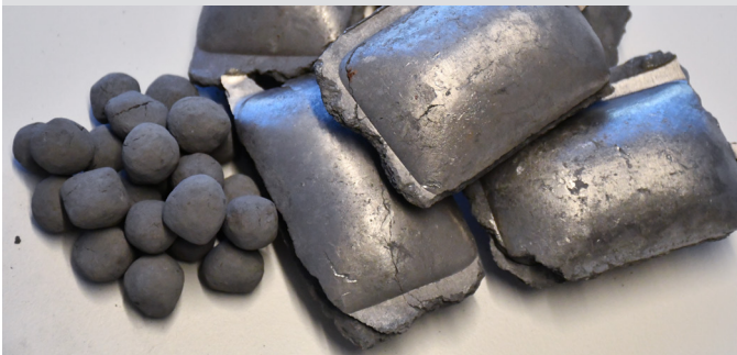
Direct Reduced Iron (DRI) pellets and Hot Briquetted Iron (HBI) briquettes.
